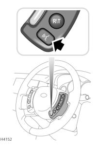
To switch on voice control, press the voice control key (arrowed) in the multi-functional steering wheel:
