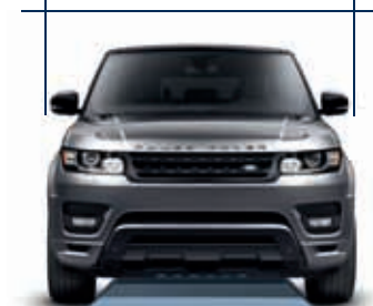
Width 81.6 inches mirrors folded Width 87.4 inches mirrors out
